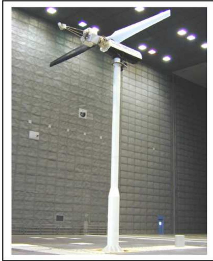
Figure 1.1. NREL UAE wind turbine mounted in NASA Ames 80 \times 120 foot wind tunnel [32]
